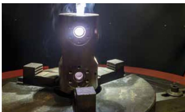
Small internal diameter welding overlays
