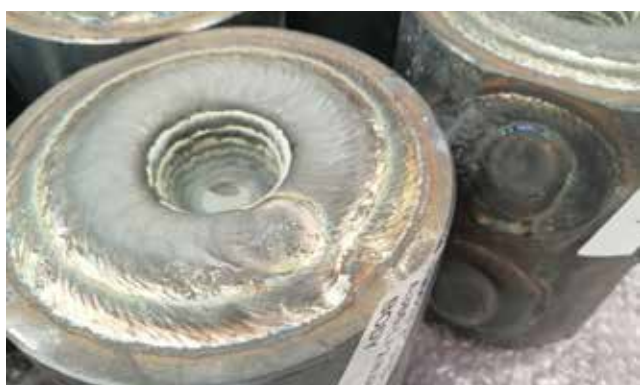
Welded overlays on chamfer/bewel
