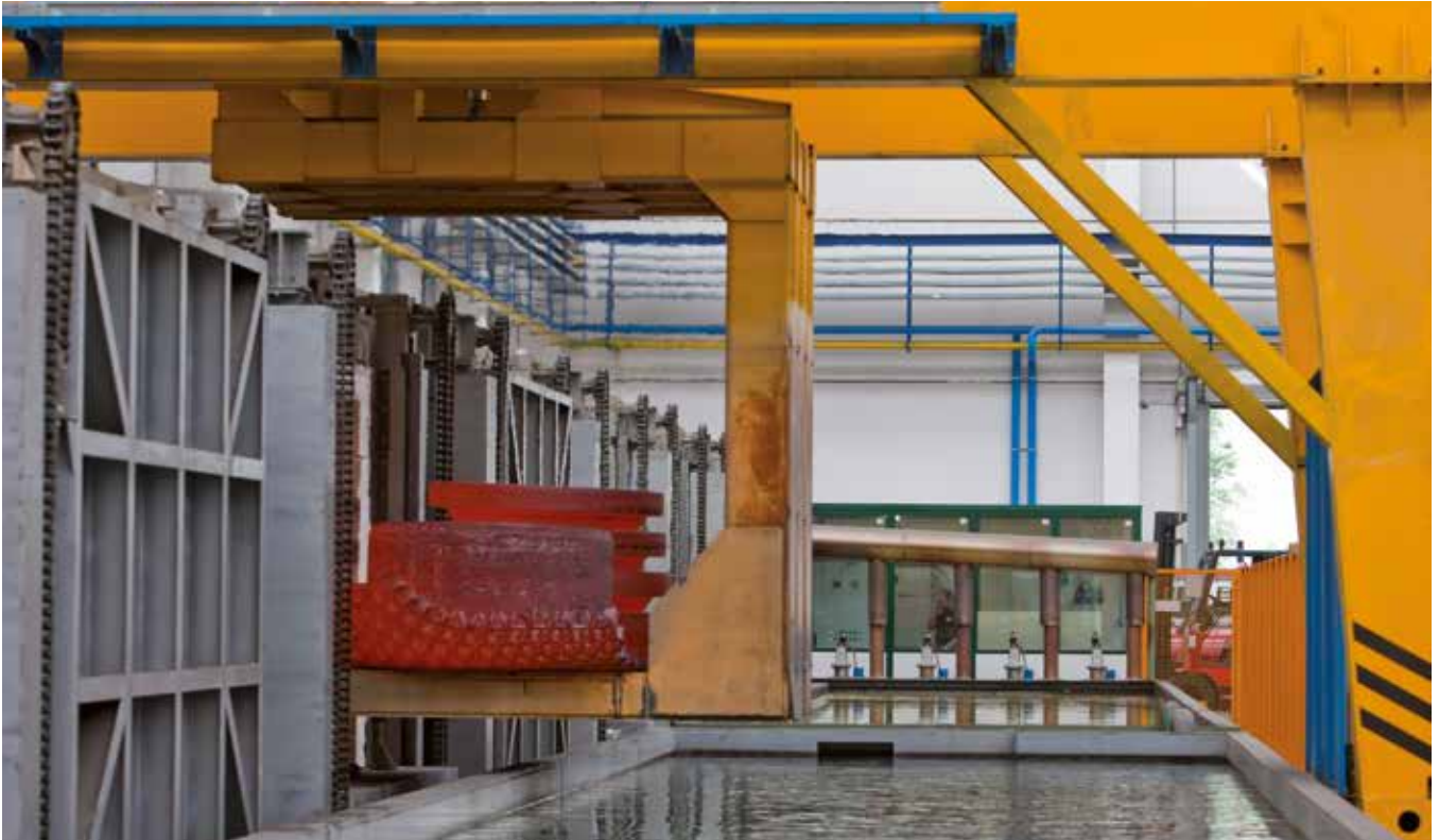
Furnace heating and water or polymer quenching
